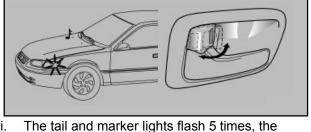
The tail and marker lights flash 5 times, the buzzer chirps 5 times and the doors lock and unlock 5 times.\*
