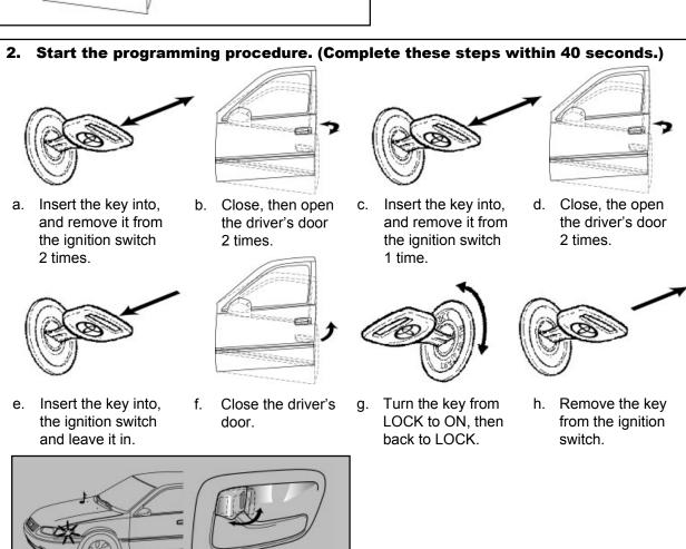
The tail and marker lights flash 1 time, the buzzer chirps 1 time and the doors
